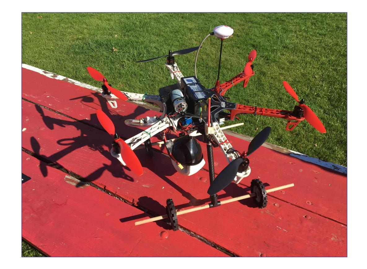
★ Low resolution downward facing Logitech webcam. Outputs video to Raspberry Pi for analysis.
